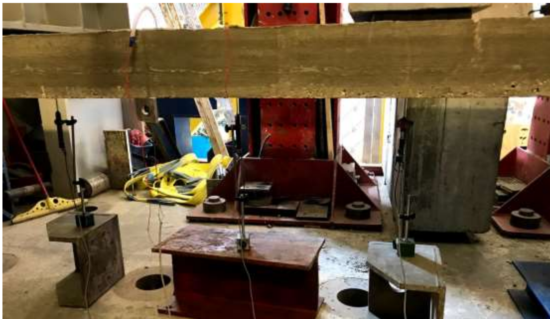
Figure 5-4 UBSR 1 with a sketch for the location of four LVDTs (top) and the LVDTs in their positions in reality (bottom)
