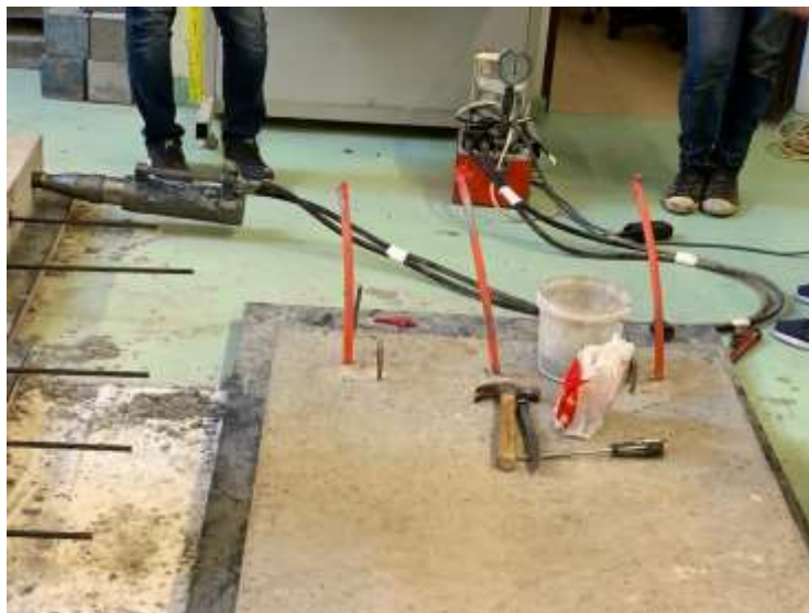
Figure 4-20 The setup of the slab specimens with an indication for the dead and live ends (All dimensions are in millimeters) (top) and the hydraulic jack connected to one of the unbonded tendon to apply the prestressing designed force (bottom)
