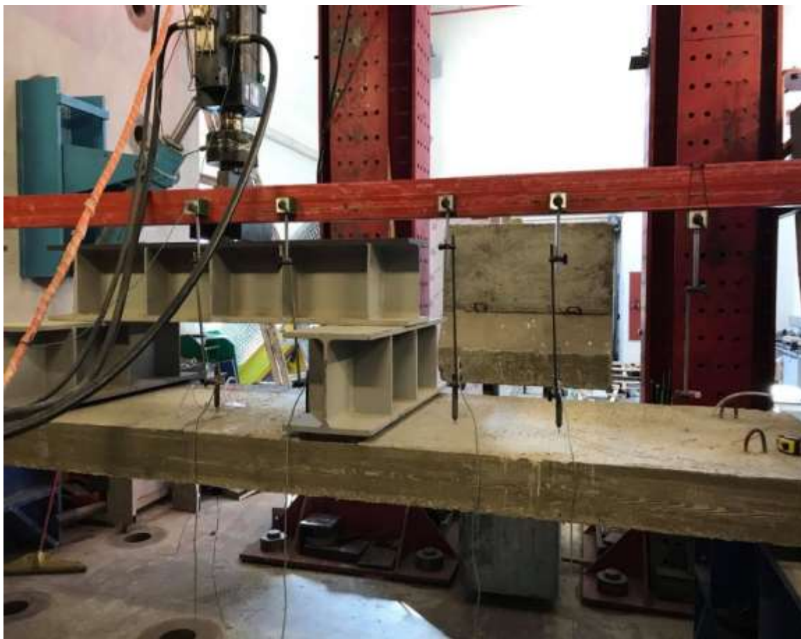
Figure 5-9 Sketch for the five LVDTs positioned for UBS1 at different locations (top) and their positions in reality (bottom)
