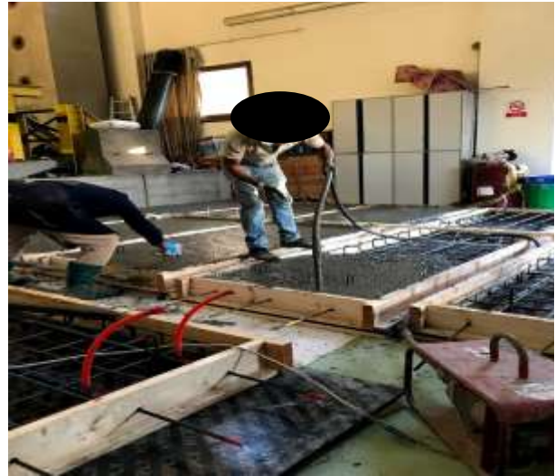
Figure 4-15 Concrete casting for the slab specimens (left) and concrete compaction and surface smoothing (right)
