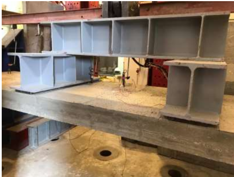
Figure 5-10 Strain gage located on the concrete top surface (top) and loading beams full set up (bottom).
