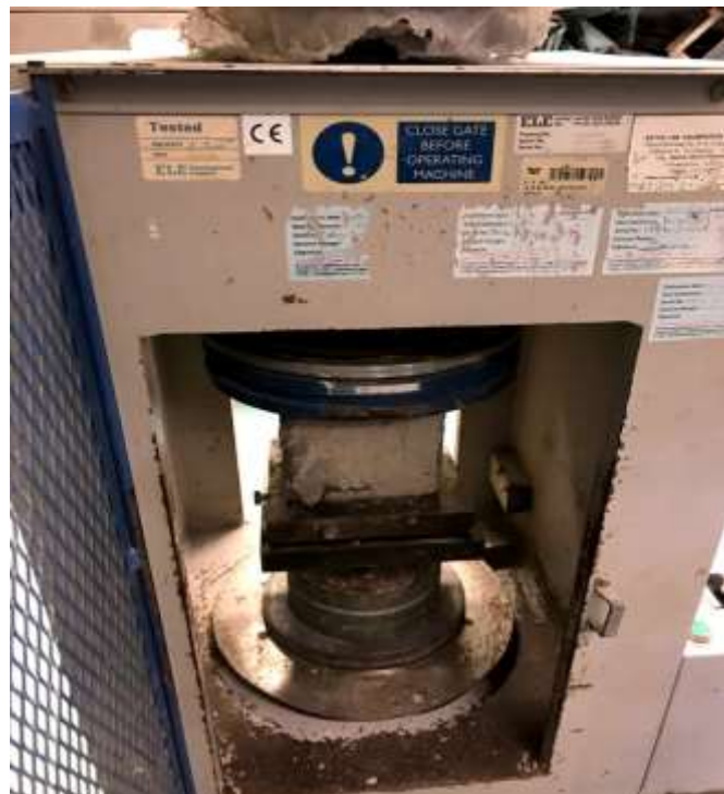
Figure 4-18 Standard concrete cube under compression load, showing cracks
