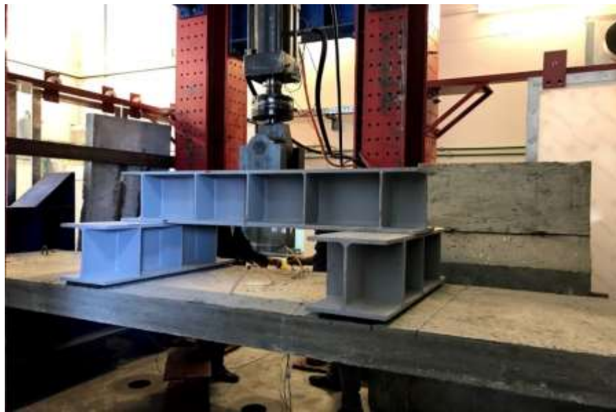
Figure 4-23 The planned setup for the tested specimens showing the locations of the loading beams and their sizes and dimensions (All dimensions are in millimeters) (top) and the setup prepared in reality at the AUC structural engineering lab (bottom)
