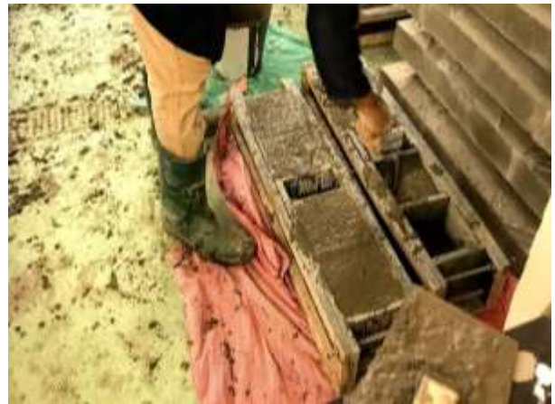
Figure 4-15 Concrete casting for the slab specimens (left) and concrete compaction and surface smoothing (right)
