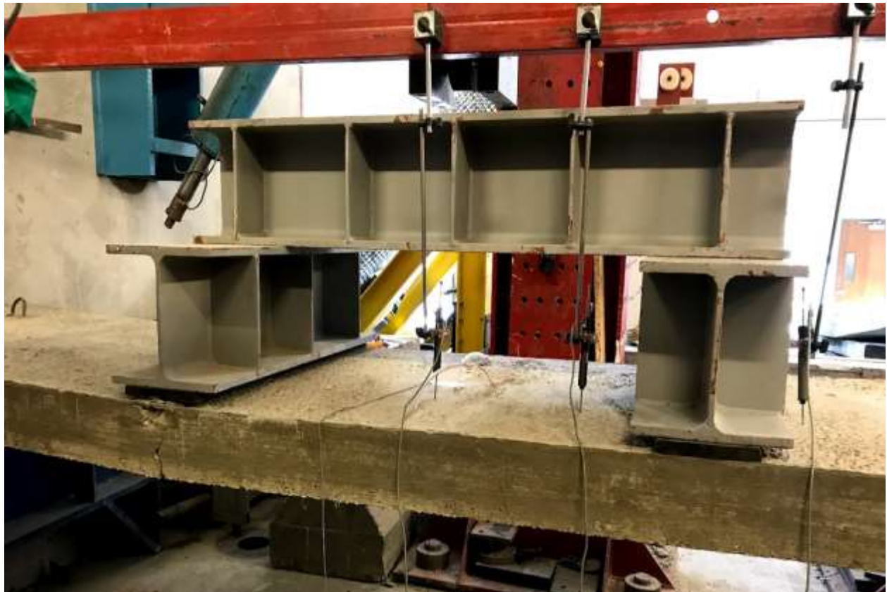
Figure 5-25 UBS2 during failure showing maximum deflection (top) and after failure and the removal of the load (bottom)
