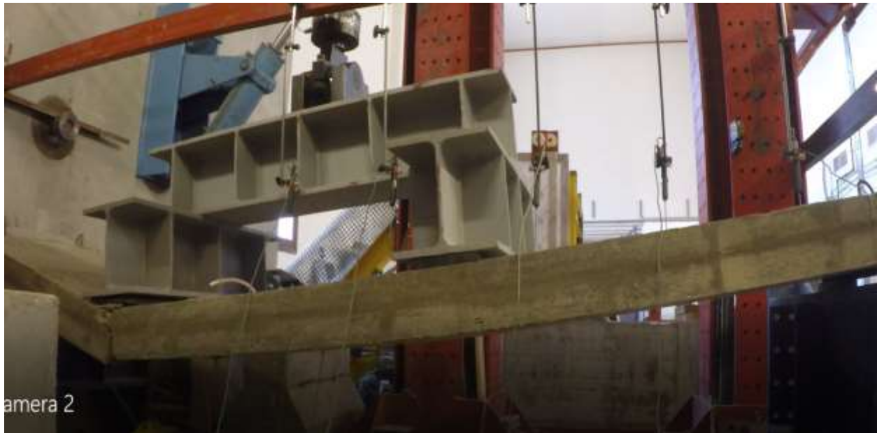
Figure 5-14 BS2 set up complete with LVDTs positioned as demonstrated and strain gages shown on the top and bottom surfaces of the concrete (top) and its failure due to the formation of one single crack underneath one of the loading beams (bottom)
