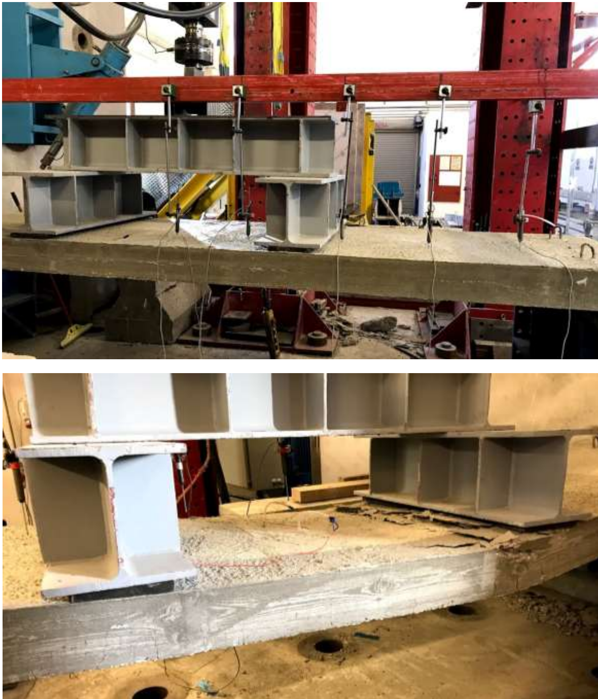
Figure 5-19 The complete set up of UBSR 2 before the start of the flexural test (top) and after failure (bottom)
