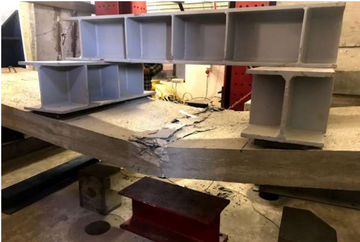
Figure 5-5 Unbonded slab without reinforcement UBSR1 after failure showing the concrete crushing ant the compression zone and the cracks formed at the tension zone
