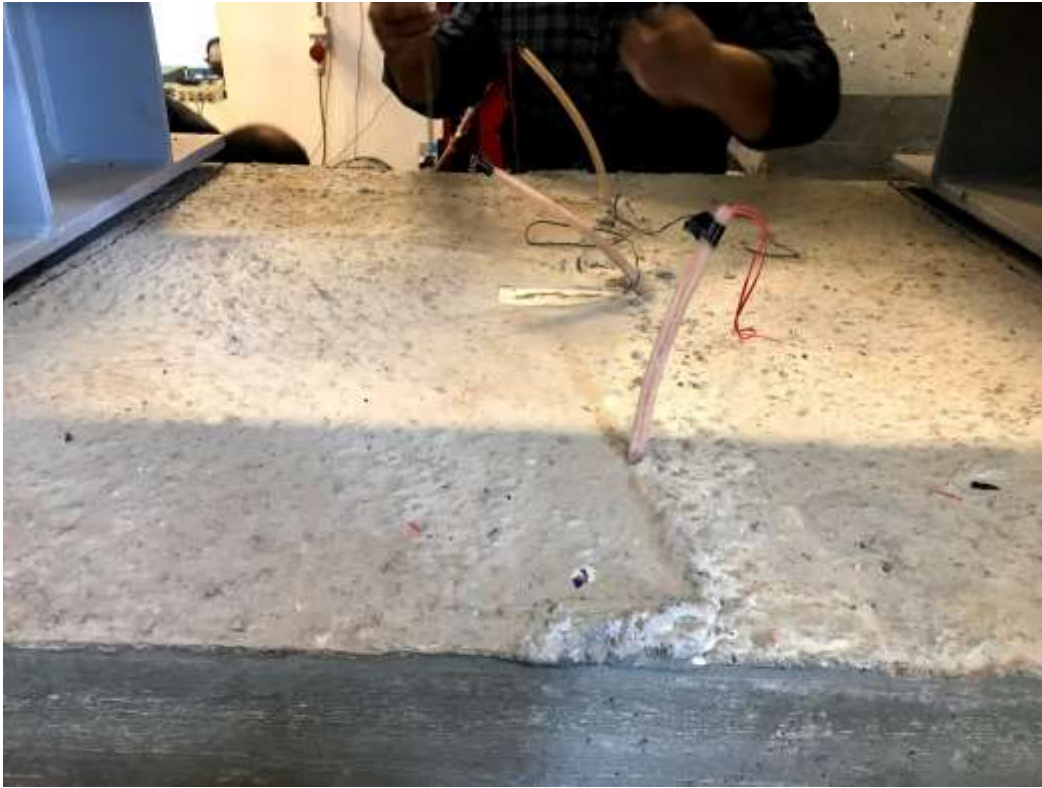
Figure 4-24 Strain gage attached to the concrete top surface
