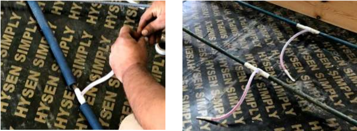
Figure 4-11 Strain gauge wires inserted inside the plastic tube (left) and strain gauges fixed on the unbonded tendons in their designed spots (right)
