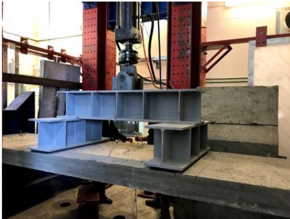
Figure 5-1 Bonded slab without non-prestressing steel reinforcement specimen BS1 before testing
