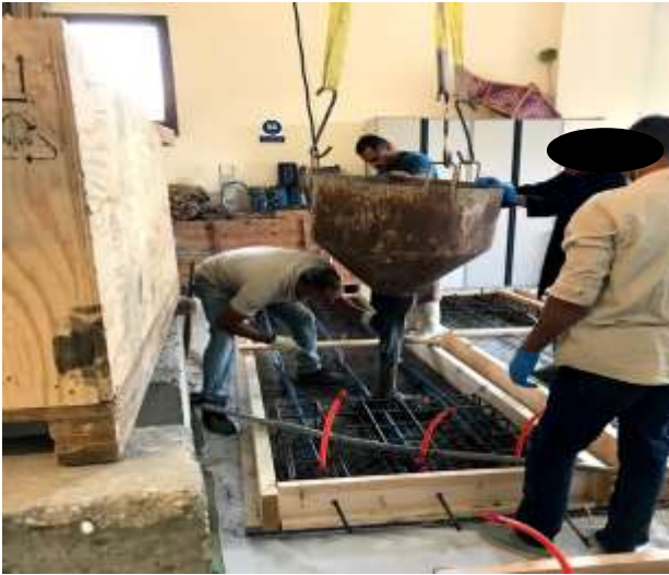
Figure 4-15 Concrete casting for the slab specimens (left) and concrete compaction and surface smoothing (right)
